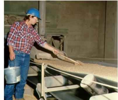
Figure 32: Sampling grain from a horizontal belt
