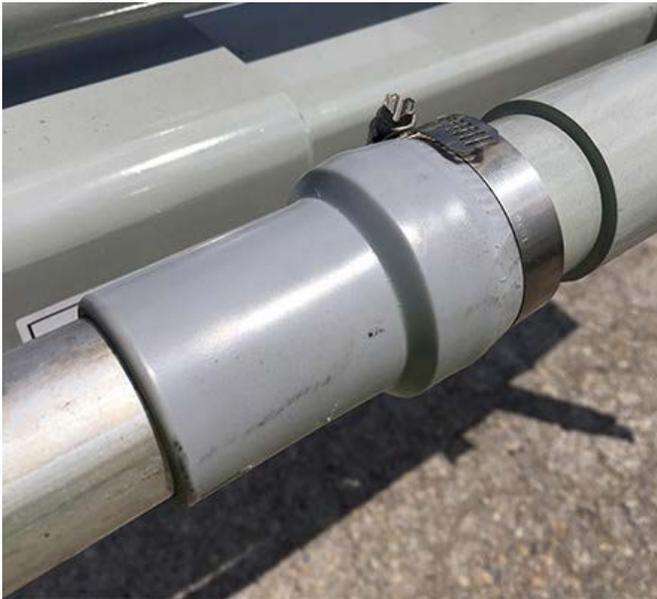
Figure 26: Rubber gasket boom sleeve
