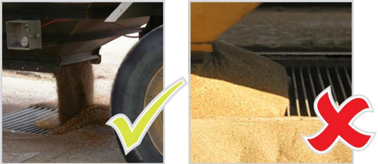
Figure 29: Manual stream sampling over an open pit
