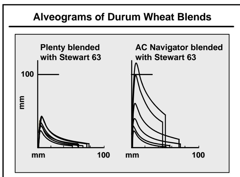
Fig. 3. Alveograph curves obtained from 100% Stewart 63 semolina, and from various blends of Stewart 63 semolina with semolina from the Canadian durum wheat varieties Plenty and AC Navigator.
